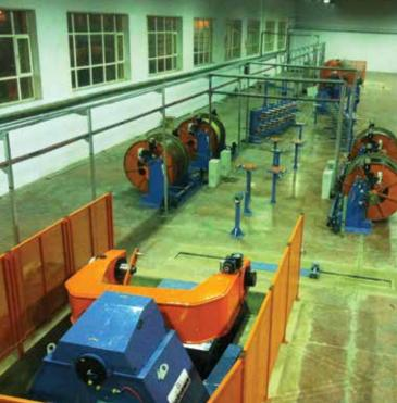
Reliable and precise armouring solutions Adjustable wire tension during operation.
